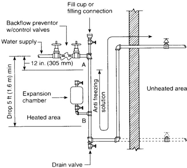
**FIGURE 14.16** Acceptable antifreeze u-loop configuration. (Reprinted with permission from NFPA 13, *Installation of Sprinkler Systems*, Copyright © 1996, National Fire Protection Association, Quincy, MA 02269. This reprinted material is not the complete and official position of the National Fire Protection Association, on the referenced subject, which is represented only by the standard in its entirety.)
