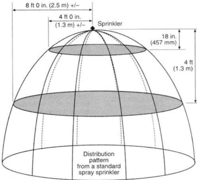
**FIGURE 14.18** Typical distribution pattern from a standard spray sprinkler. (Reprinted with permission from *Fire Protection Handbook*, Copyright © 1997, National Fire Protection Association, Quincy, MA 02269.)
