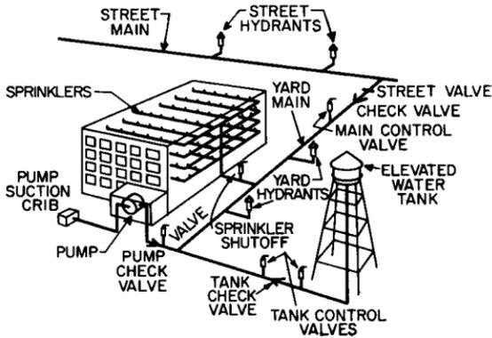
FIGURE 14.21 Water-supply piping for sprinklers.
