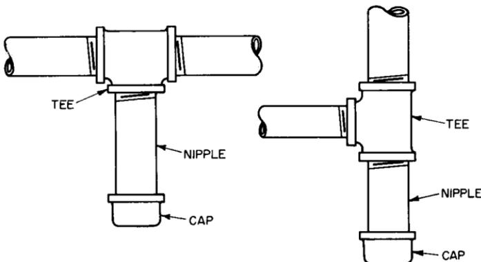
FIGURE 14.13 Drips for gas piping.
