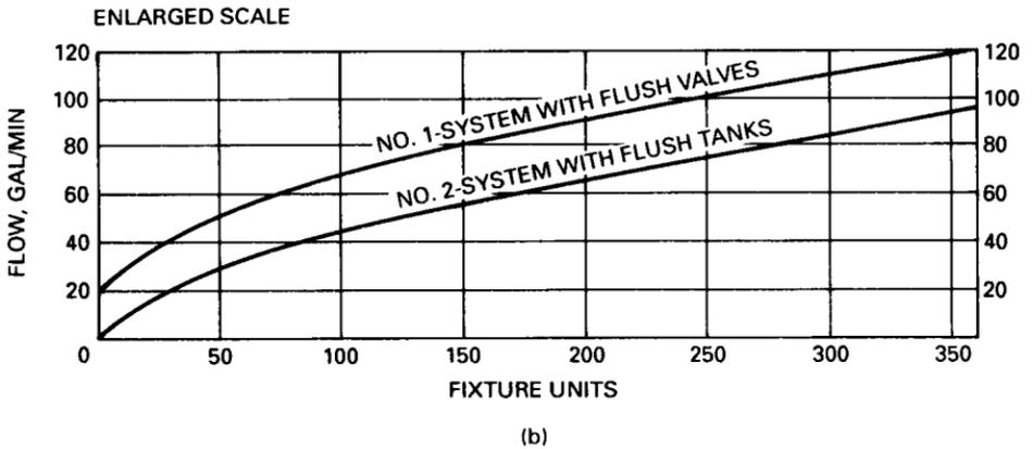
FIGURE 14.4 Estimate curves for domestic water demand. (a) The number of fixture units served determines the rate of flow. (b) Enlargement of the low-demand portion of (a).
