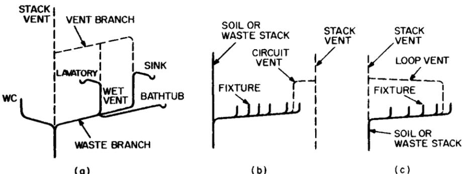
**FIGURE 14.11** Venting of waste branches: (a) wet venting of bathtub drainage pipe; (b) circuit venting, and (c) loop venting of a battery of plumbing fixtures.
