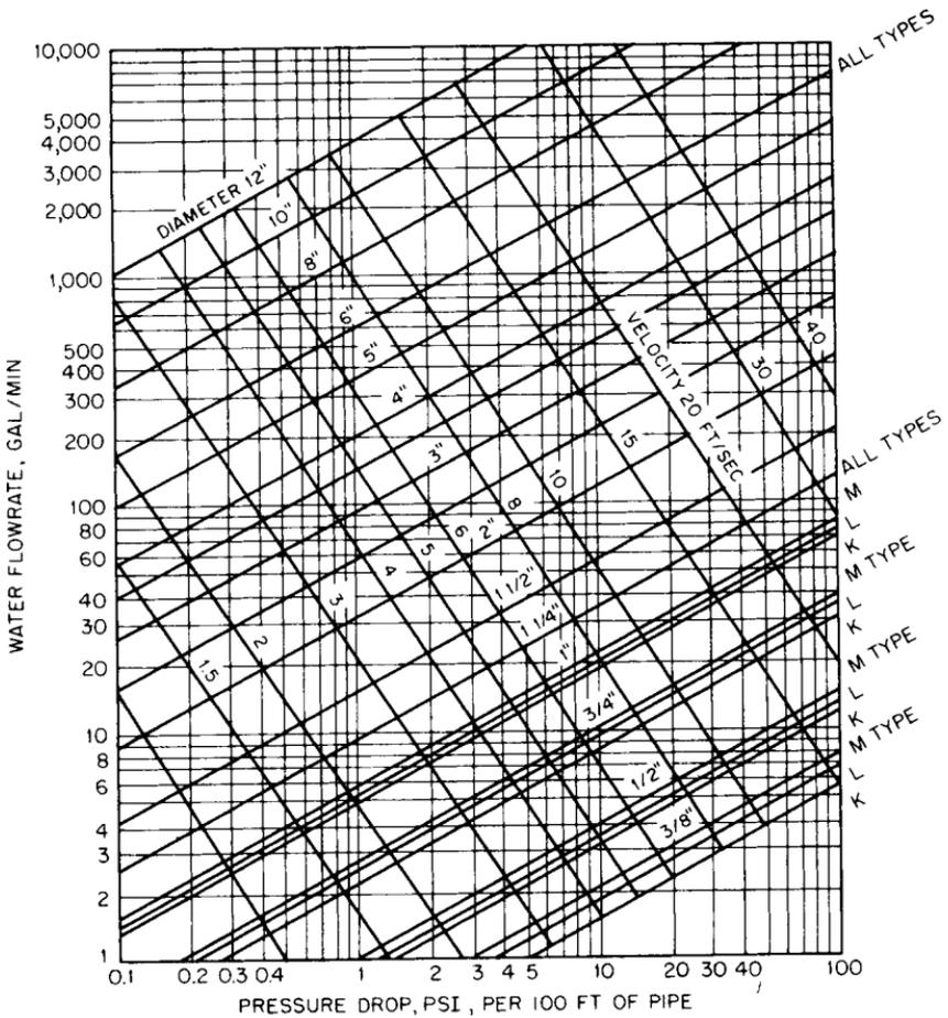
**FIGURE 14.5** Chart for determination of flow in copper tubing and other pipes that will be smooth after 15 to 20 years of use.
