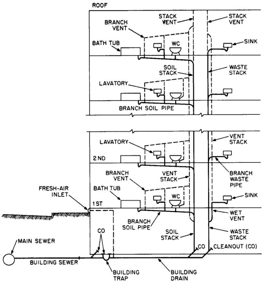
**FIGURE 14.9** Wastewater-removal system for a multistory building. (Reprinted with permission from F. S. Merritt, "Building Engineering and Systems Design," Van Nostrand Reinhold Company, New York.)
