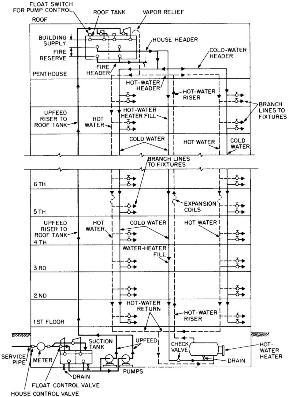
**FIGURE 14.2** Down-feed water-distribution system for a tall building. (Reprinted with permission from F. S. Merritt, "Building Engineering and Systems Design," Van Nostrand and Reinhold Company, New York.)
