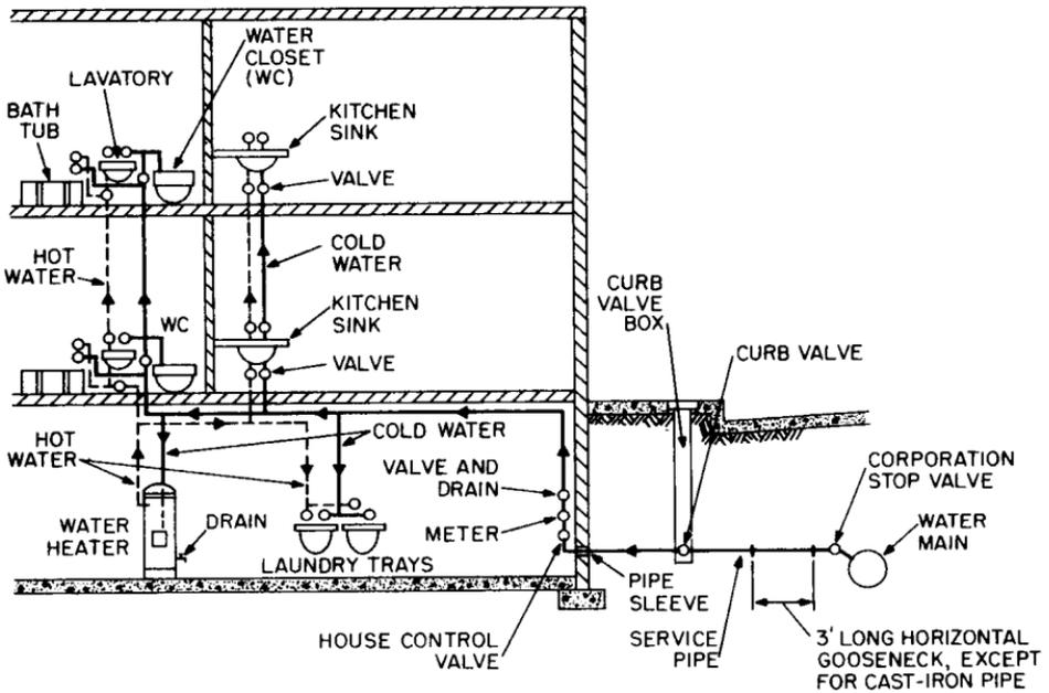
**FIGURE 14.1** Up-feed water-distribution system for a two-story apartment building. (Reprinted with permission from F. S. Merritt, "Building Engineering and Systems Design," Van Nostrand Reinhold Company, New York.)
