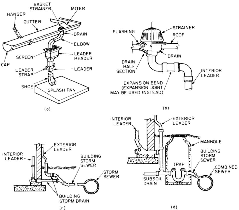
**FIGURE 14.10** Elements of a storm-drainage system: (a) roof gutter, exterior leader, and splash pan; (b) roof drain and top portion of interior leader; (c) piping to a storm sewer; (d) piping to a combined sewer. (Reprinted with permission from F. S. Merritt, "Building Engineering and Systems Design," Van Nostrand Reinhold Company, New York.)
